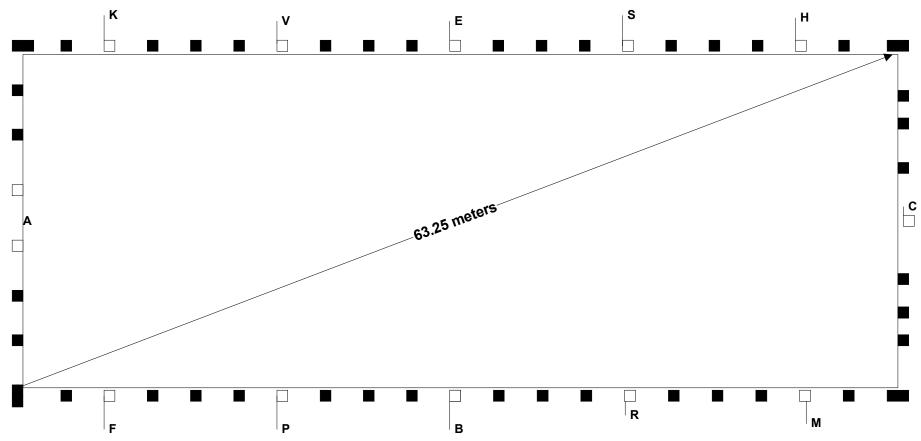
Long Sides 20/3 meter rails – start with one at corner, place black pylon every 3 meters. white pylon at letters.
